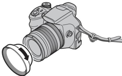
Mount the Wide conversion lens by screwing in the direction of arrow.
